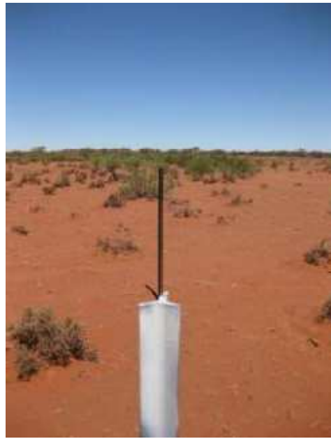
Figure 11 White paint to guide photo orientation
