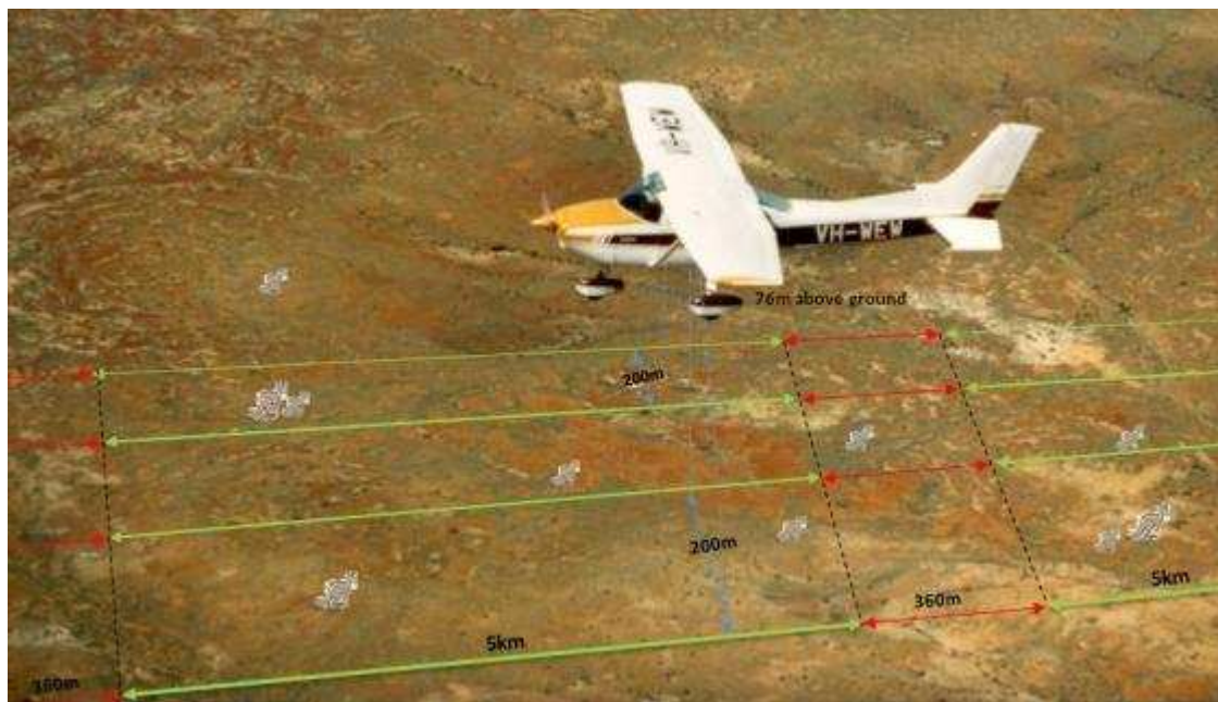
Figure 6: Strip transect sampling from fixed-wing aircraft
