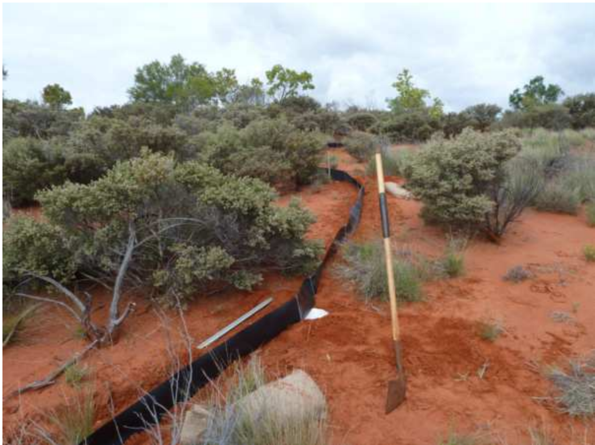
Figure 2 Bucket trap design – Site Old Road dune
